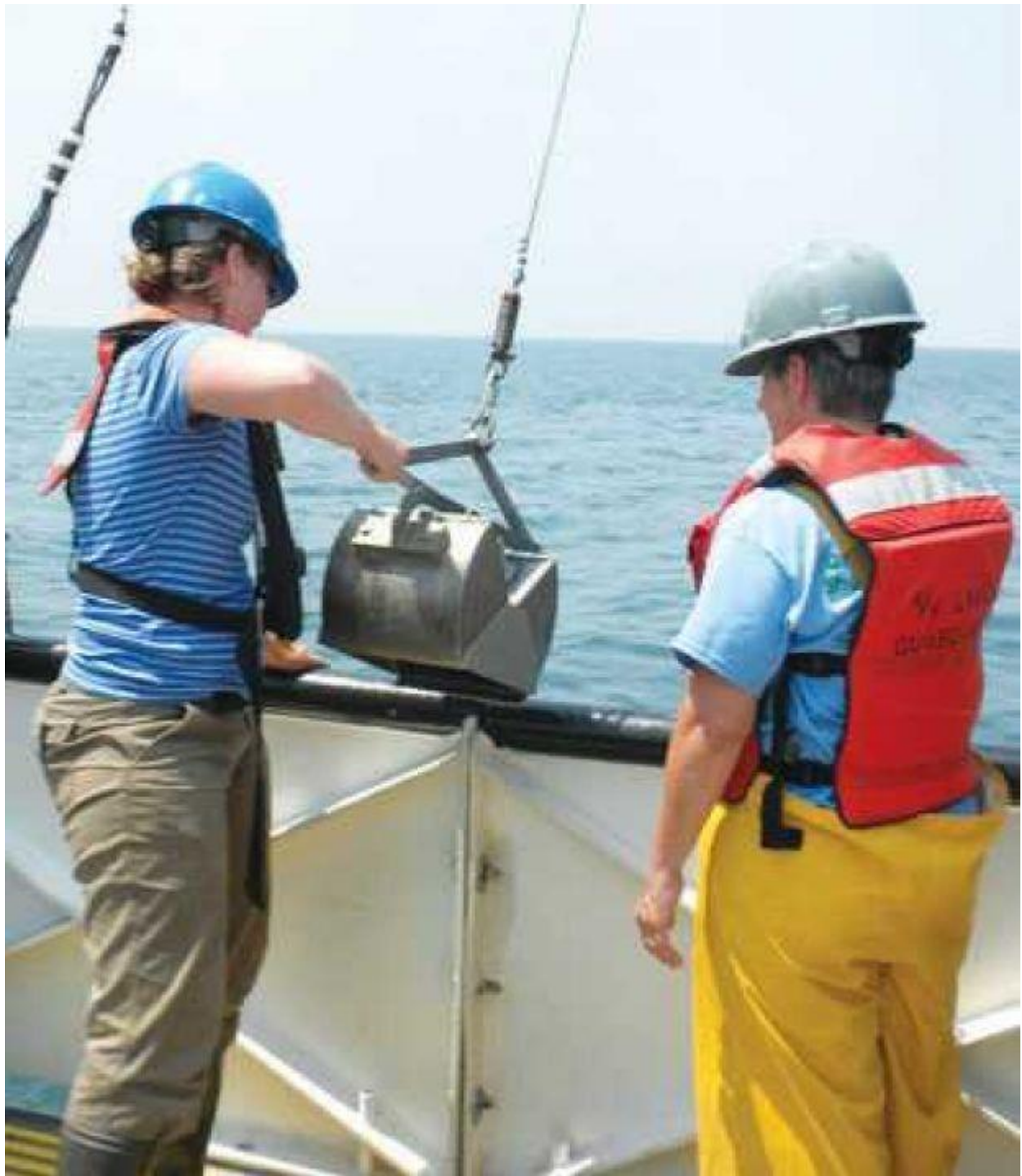
A researcher aboard the research vessel Lake Guardian prepares the ships ponar for a grab below the surface of Lake Ontario as Cicero-North Syracuse High School teacher Kim Linkinhoker looks on. The ponar collects mud samples for biological studies of the lake's benthic animals, including worms, snails, crustaceans and midge fly larvae. Submitted photo.
