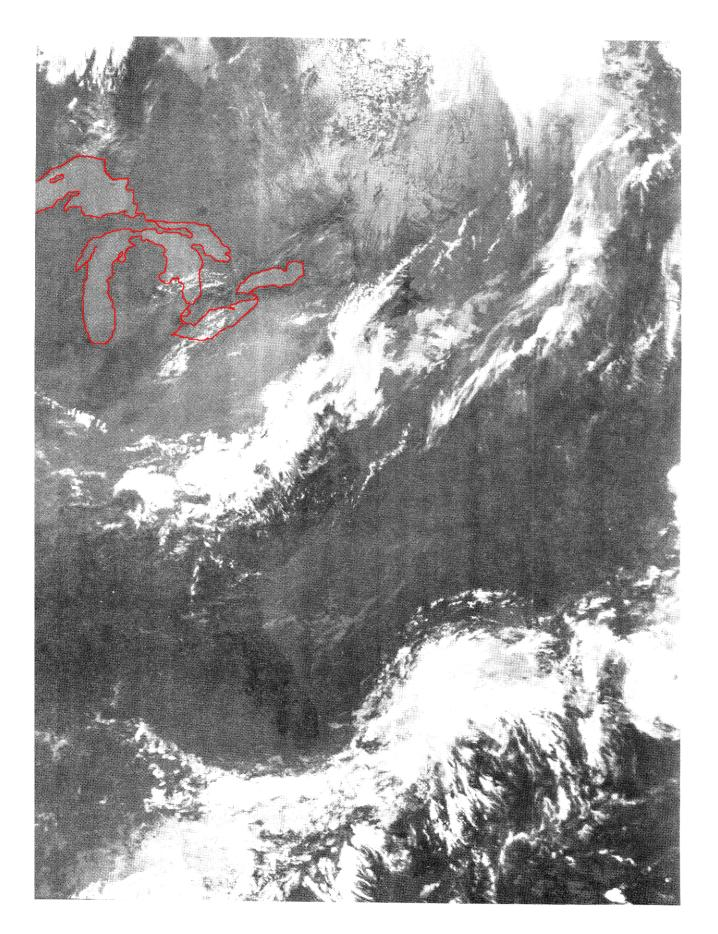
Infrared images show warmer areas as darker, colder areas as lighter. Notice the high clouds which appear as bright white patches. In June the lakes are colder than the land and so appear lighter in the infrared image.
