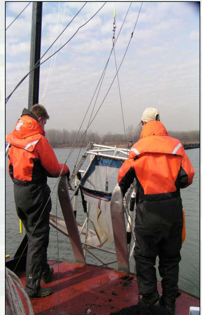
epibenthic sled-mounted 0.5-m plankton nets (0.5-mm mesh)
