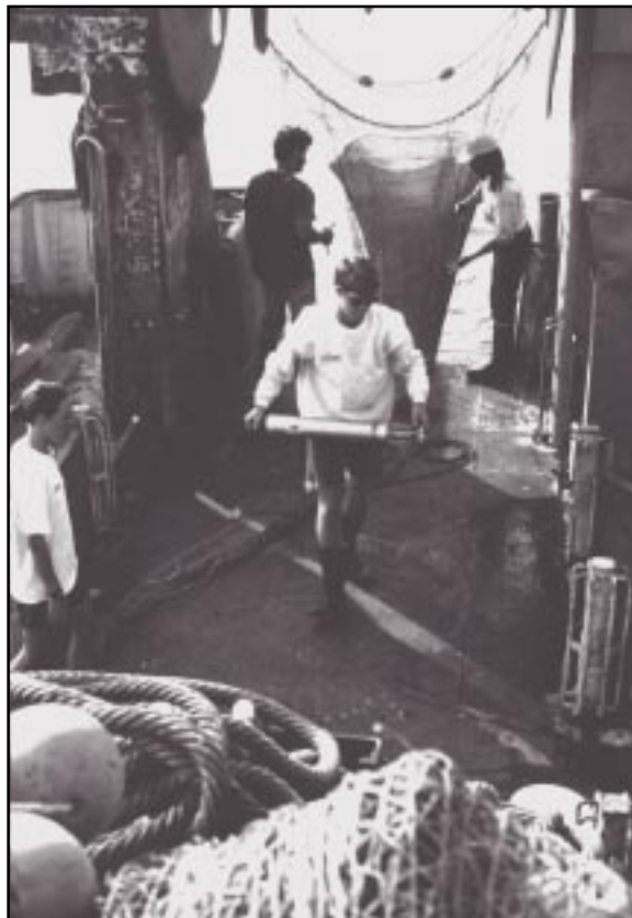
Aboard the F/V Illusion , graduate student Brian Steves collects conductivity, temperature and depth data using a CTD instrument. Biological sampling was conducted using 6-foot beam trawls. Photo by Mark Malchoff
