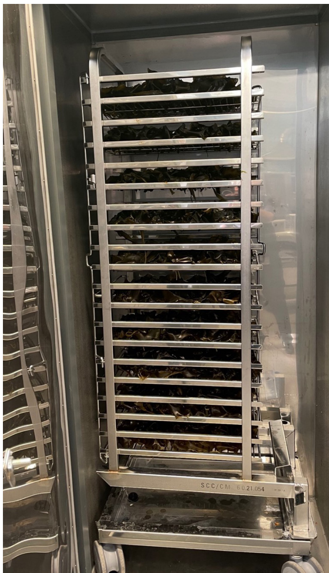
Commercial Air Dryer: Nyle Systems FD 2.5 Food Dehydrator (discontinued but new models available)
