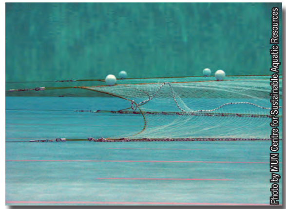
The November trawl workshop featured trawl scale models such as this one being tested in the Memorial University of Newfoundland flume tank, the largest in the world.
