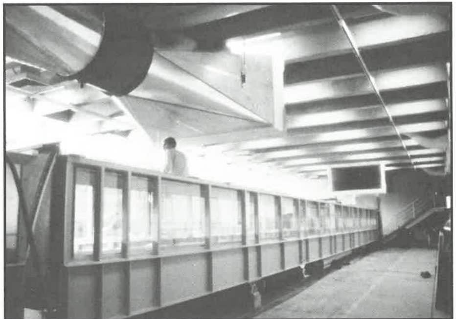
The Tilting Wind-Water Tunnel (TWWT) in the Defrees Hydraulics Laboratory at Cornell University. TWWT is used to simulate wind/water interaction conditions in the natural environment. Photo courtesy Dr. Chia-Ren Chu.
