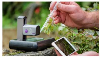
Water sample is deposited under a special microscope that is synced to the user's cellphone to take pictures. The photos are uploaded to the BloomOptix server for diatom identification and cell count analysis. Photo: BloomOptix
