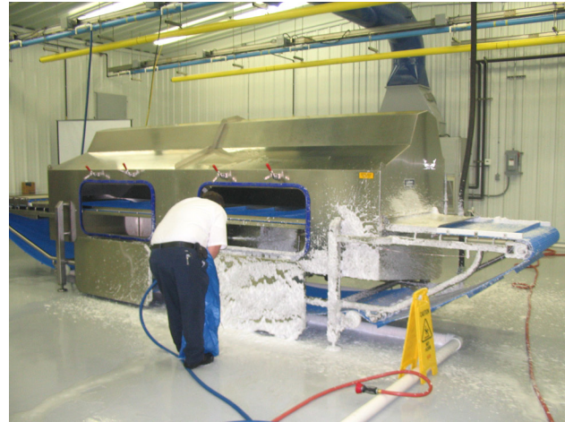
Back to Basics: Seafood businesses across New York are utilizing a new web-based, on-demand, low-cost NY Sea Grant training program to train employees in the application of basic food safety concepts and practices (above: foam cleaning of processing equipment).
