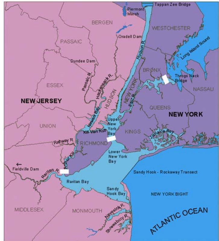
The waterways surrounding New York City could potentially be protected from coastal flooding with three barriers (shown in white) located from west to east at Perth Amboy, NJ, the Narrows and the Upper East River.
