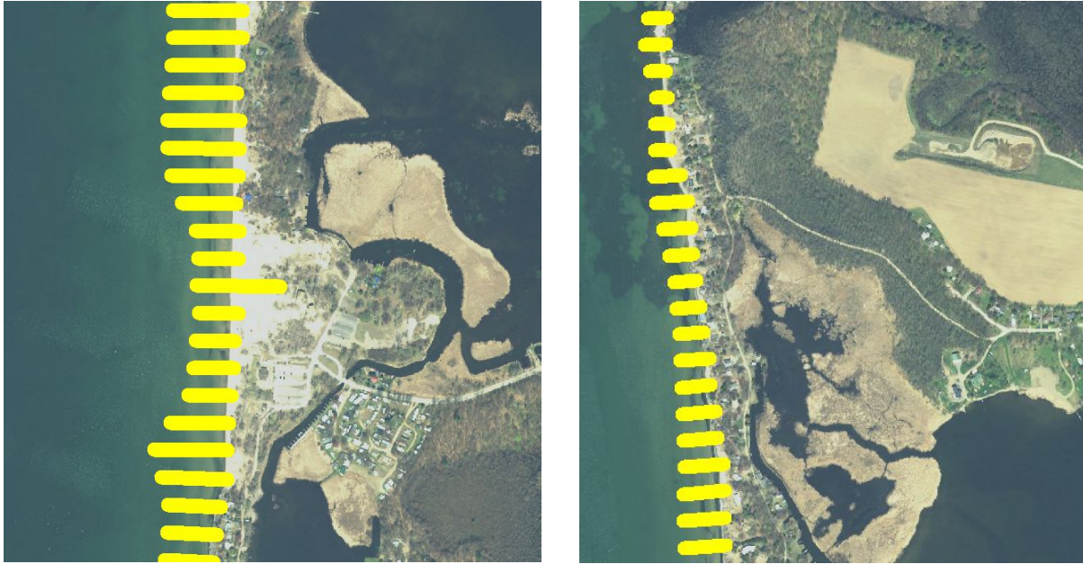
Figure 43: Dune blow-out showing lower shoreline retreat of ranging from 60 - 70 meters (left). Northern extent of study area with lower shoreline retreat ranging from 10 to 50 meters (right).
