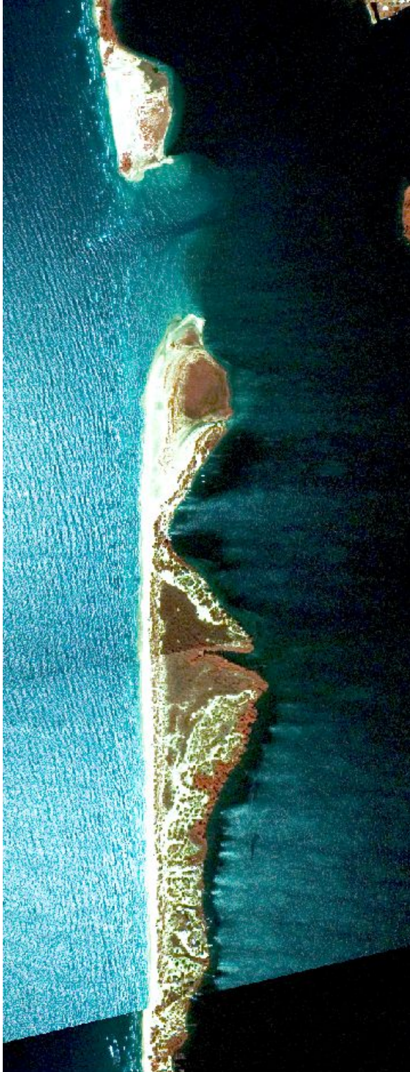
Figure 66: A return of higher lake levels in 1983 flooded low areas of new sand bars adjacent to the inlet which now was 1500 feet wide, with a small deeper channel at its center.
